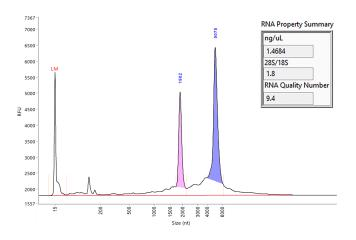
**Figure 1.** Total RNA sample separated using the HS RNA kit (p/n DNF-472) on the 5200 Fragment Analyzer system. The RNA Property Summary offers further insight into individual samples, reporting the RQN, concentration, and rRNA ratios.
