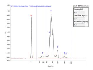
**Figure 2.** Small RNA sample separated using the Small RNA kit (p/n DNF-470) on the 5200 Fragment Analyzer system. Small RNA and microRNA concentrations and the percent mircoRNA are reported in the RNA Property Summary.
